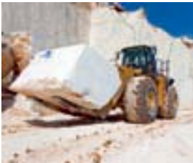
A large block of marble is carried away from the quarry face for processing in the nearby factory.
